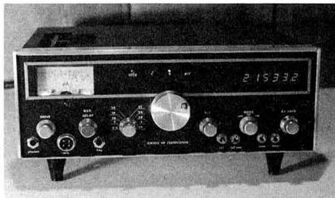
Front view of the all-band version of the transceiver. Amendments include new bandswitch markings and i.e.d. synthesizer lock indicator
